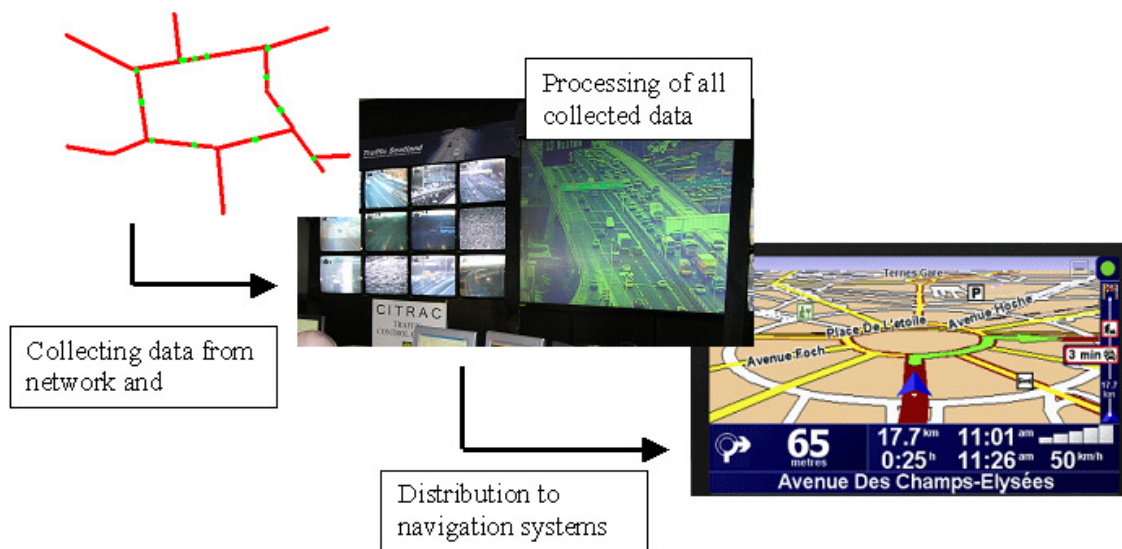
Figure 2-10 Processing of measured travel times
